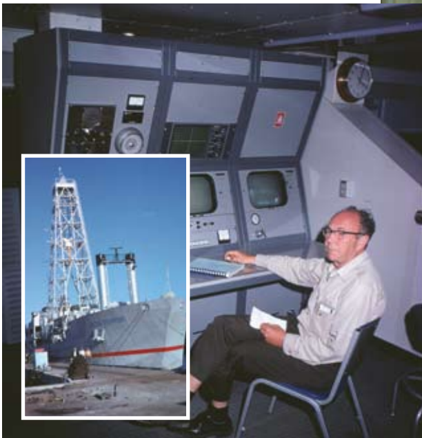
Insert: The all-aluminum survey vessel Alcoa Seaprobe . Search equipment and a giant clamshell were operated through an open well ("Moon pool") in the middle of the ship.
