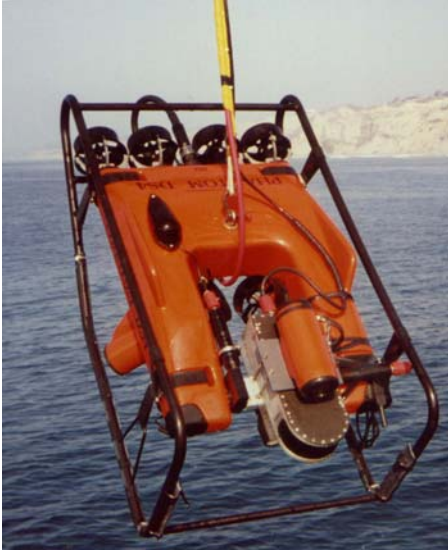
EODTC Phantom HVS4 with multibeam sonar
